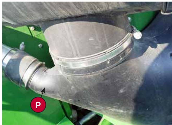
19. Late model S600 or S700 Series Combines have a secondary inlet (P)
