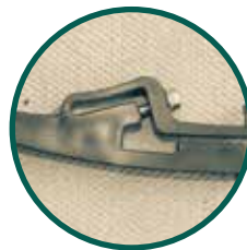
Connect to firmer bracket Secure seed firmer connection. 2A: When tightening the FR200 screw back off two turns after screw has hit firmer.
