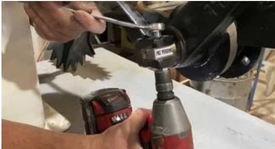
Reattach the depth adjustment arm securely
