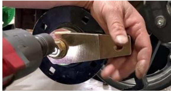
Torque the flange nut to 120ft/lbs
