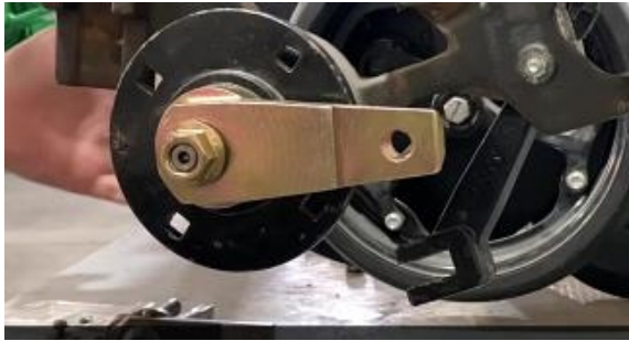
Install the flange nut
