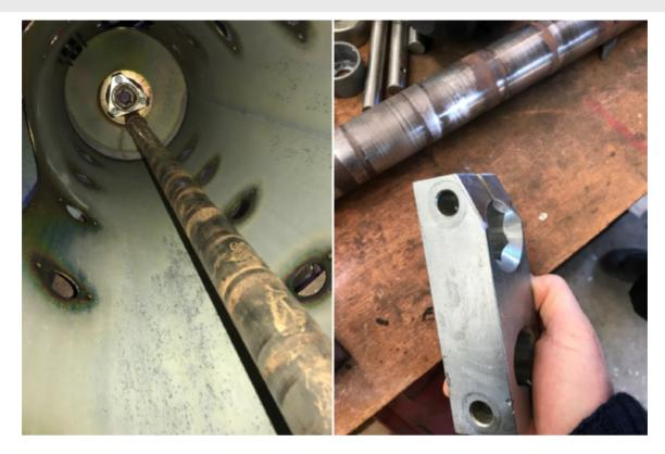
• Install the new retractable fingers (supplied) to the crankshaft using the original and supplied finger holders.
