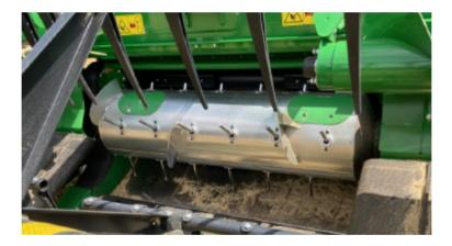
**IMPORTANT:** The correct orientation of the retractable finger timing mechanism is critical for correct performance of your iPaddock Typhoon feed drum. When positioned correctly, the fingers should be fully extended near the forward horizontal position when the John Deere timing adjustment lever is in mid range. This must be checked once the IPaddock Typhoon has been installed.
