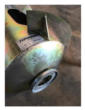
• Assemble the original hex clamped ends to the original crankshaft, inside the iPaddock Typhoon drum.
