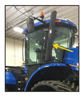
Most MY23 and up Tractors with OEM air intake tube part number 51642004 or 48065751.
